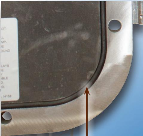
Nitrile (BUNA-N) "O" ring gasket is located inside the bolt circle for wet locations, Type 4 & IP66
