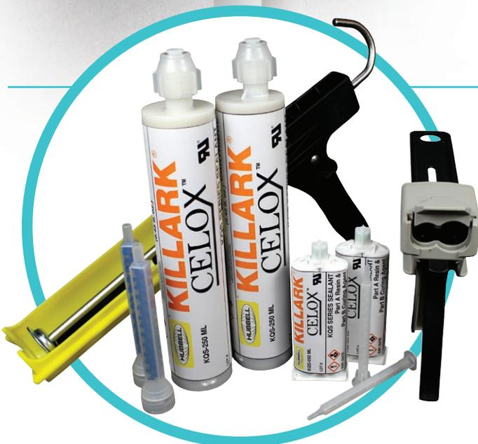
CELOX™ QoS Series is an alternative quick sealing compound used extensively for sealing conduit to prevent the spread of explosive gases and vapors. It is a two part epoxy resin that is self-mixed when pushed through a patented static mixing nozzle. CELOX™ requires no mixing, measuring, stirring, or pumping prior to pouring a seal.
